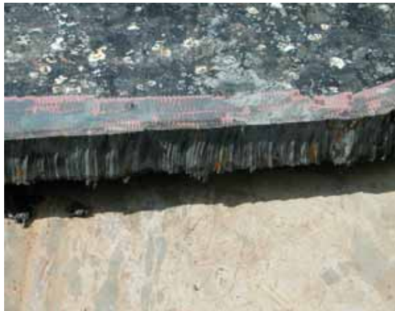
Fig.9 The plasma cut edge.
