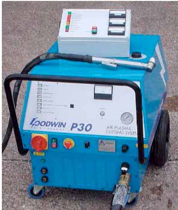
Fig.6 Power unit with torch and supervisor's control.
