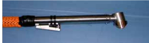
Fig.7 The new PTU (Underwater) torch
