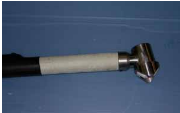
Fig.4 Standard torch with grounded body and fitted with guide ring. The handle is GRP.
